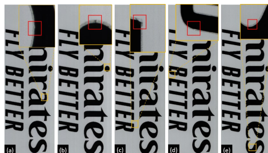
Figure 5 Defect examples (a)Less ink (b)More ink (c)Glue off (d)Less glue (e)More glue
